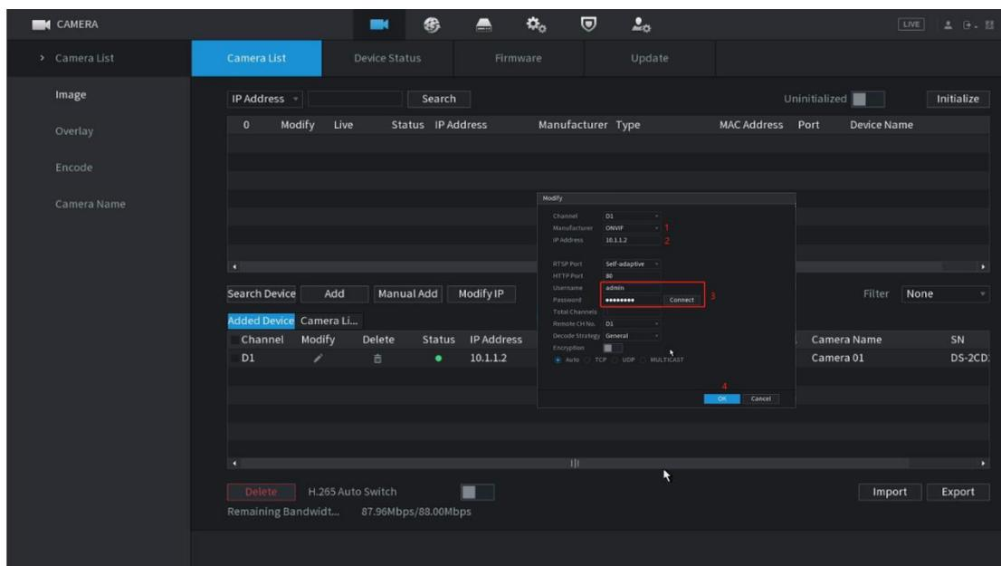
PS:When the camera status is displayed in green, the camera is successfully connected. If it is displayed in red, there is an error in the connection. Follow steps 1-5 to check whether the difference between the camera and the nvr is set correctly.
