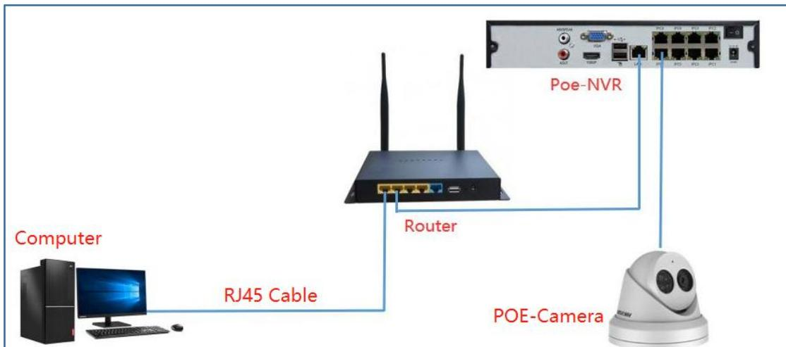
6、 Right mouse button--Main Menu -- CAMERA -- click "Manual Add" -- 1. Select the "Onvif" protocol -- fill in the camera's modified IP address -- 3. Fill in the camera's IP address, and click "Connect" -- click "OK".
