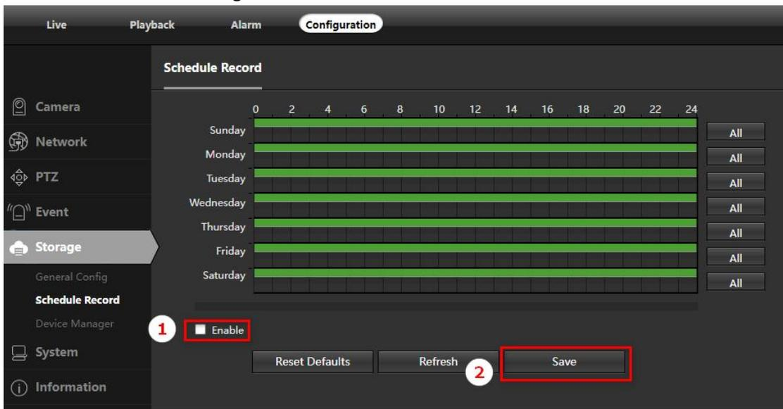
Enable intelligent detection - Trigger recording and snapshot -Set the trigger time - Save
